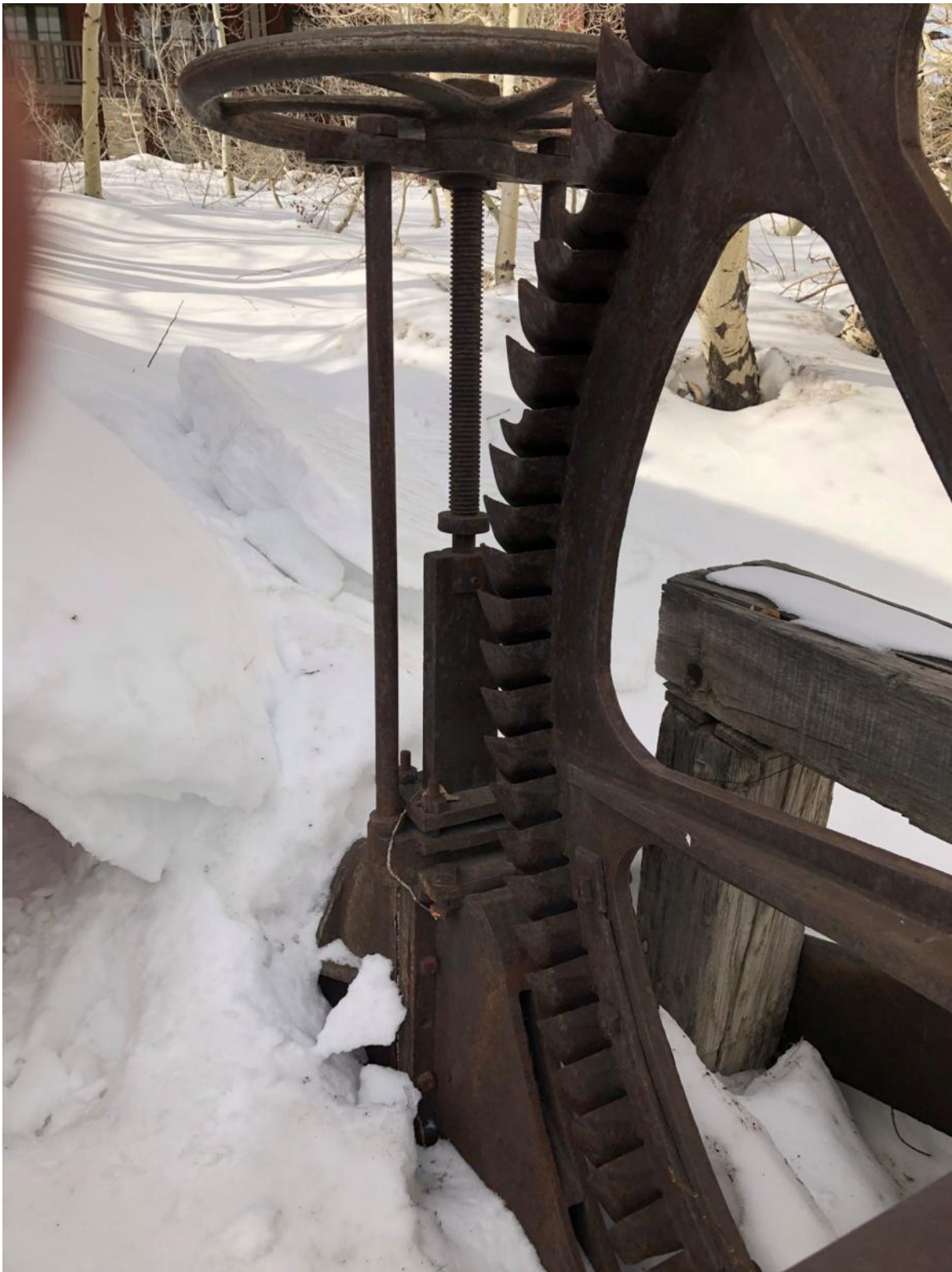
The hand wheel allows the jet of water to be adjusted and stopped.
